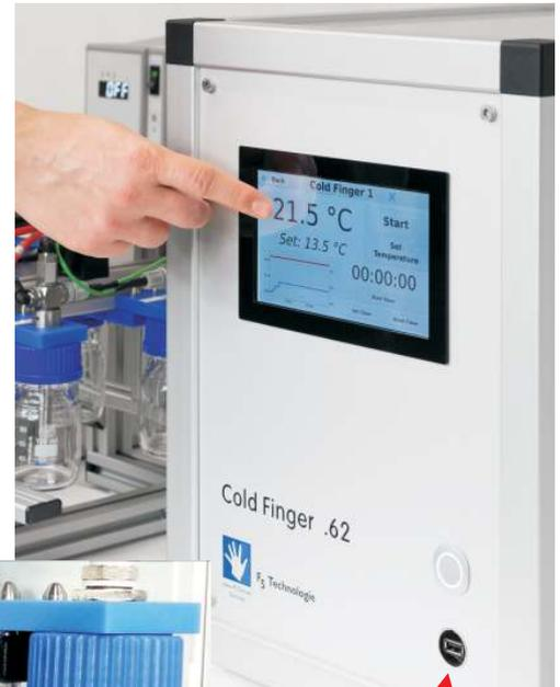
Front side USB port for data and test settings storage
