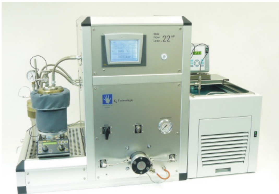
High Pressure Wax Flow Loop: 200 bar (3000 psi)
