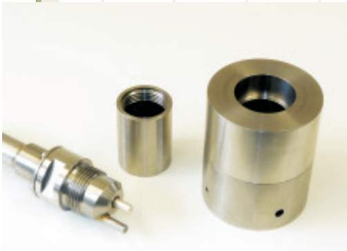
Sample containers for sample volumes of 1.0 ccm (left) and 0.5 ccm (right).
