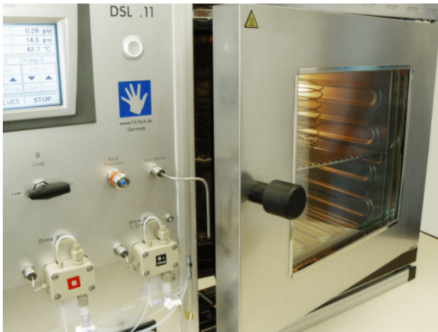
Glass door for permanent visual control of heating and test coils
