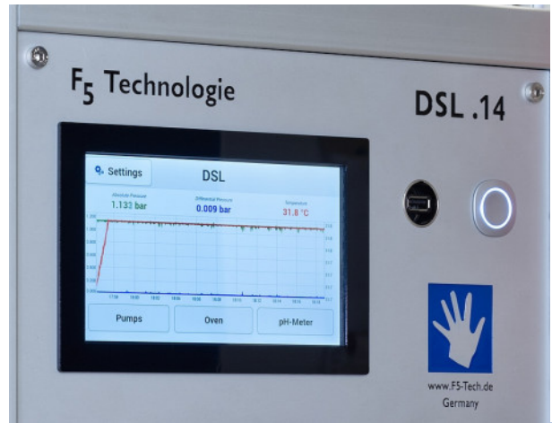
PLC with colour touch screen and big data display
