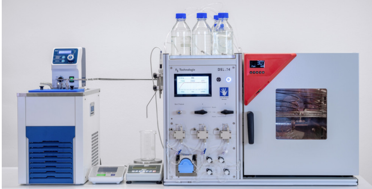
Cooling options: by liquid bath or by cooled air inside the oven
