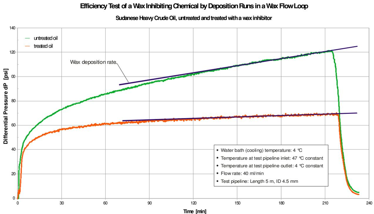
These are two basic test results: Wax deposition of an untreated oil (green) and the same oil treated with a wax deposition inhibiting chemical (orange). Both curves stabilize within the first 10 to 15 minutes. Then, the curves develop differently, which leads to the following conclusions:
