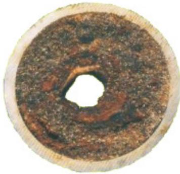
*Lateral cut of a pipeline with extreme paraffin deposition*
