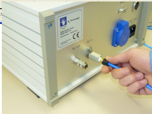
Pressure inlet up to 200 bar for gas bottle connection (field application)
