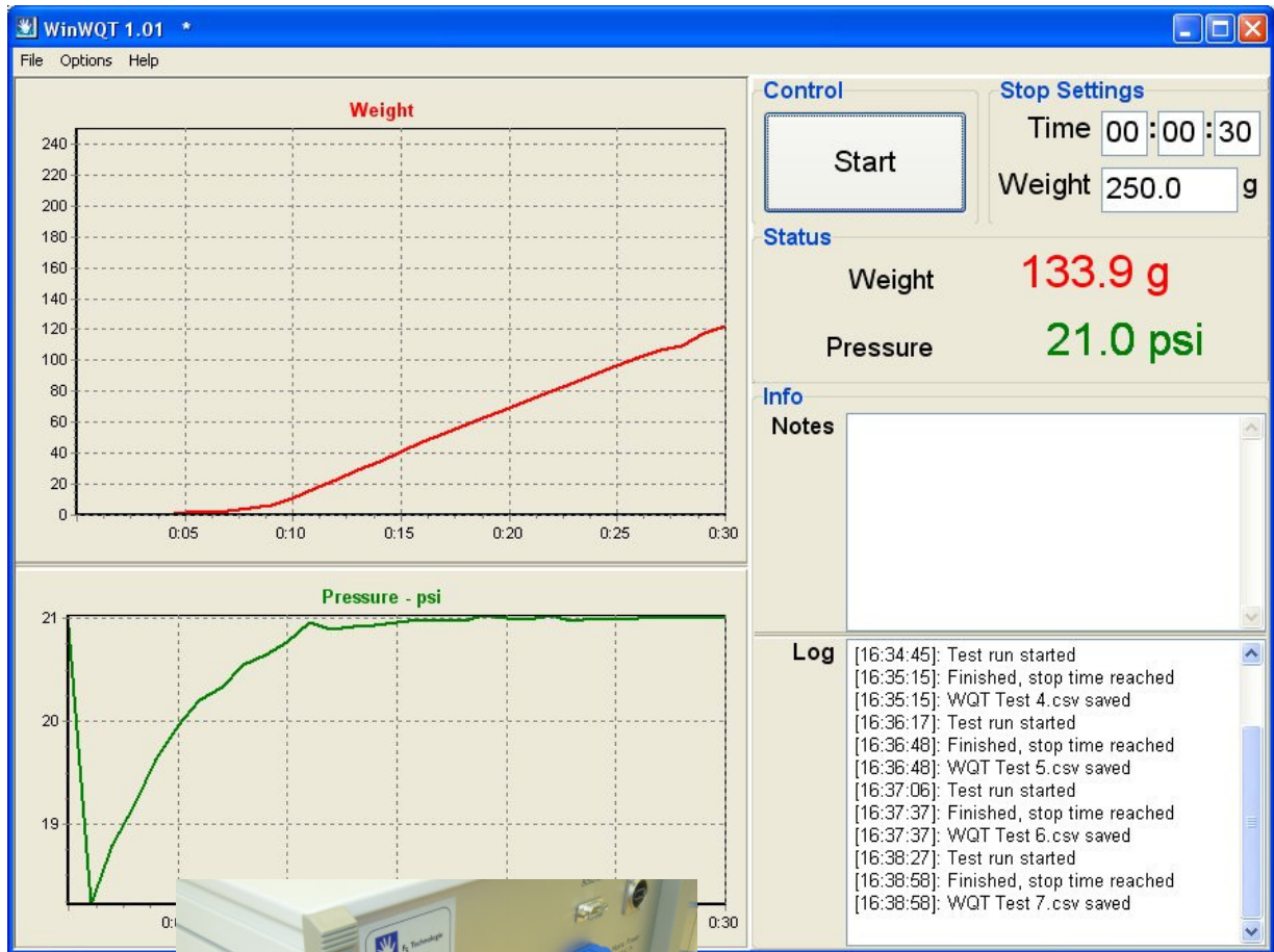
Automated measurements with WinWQT control and data visualisation software
